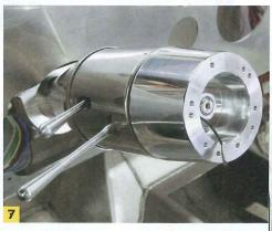
5 We'll finally be able to steel the same didn't around the shop! The old column didn't We'll finally be able to steer the Scrambler have a joint/coupling that mated to the custom steering box, so it was a major pain trying to push the Jeep around. The billet joints are machined from aircraft steel and use sealed needle bearings, which should be durable enough for years of abuse in the CJ.
