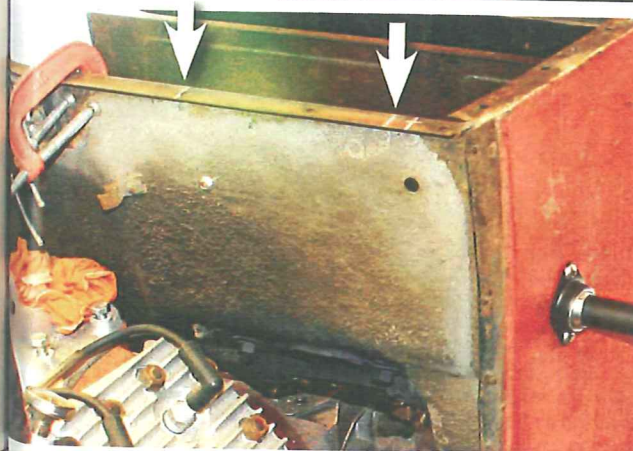
One thing I did notice though was the large diameter holes fell flush with the edge of the firewall flange. That area would have to be trimmed slightly larger than the width of the master cylinder so that it will sit flush and sandwich the firewall between it and the pedal bracket. (The arrows show the marks on the flange where it'll need to be trimmed.)
