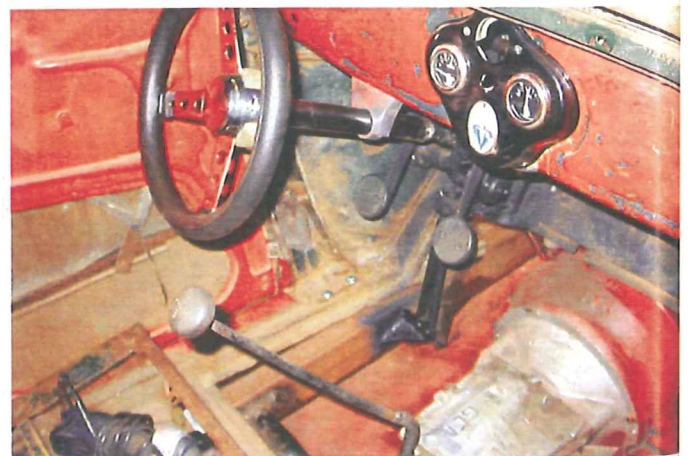
Not too bad for a weekend out in the garage. The setup seems to work just fine, and as soon as I run down and grab a clutch slave, some hard line, and a clutch disc I'll tackle the balance of the clutch and brake plumbing and assembly. Finding and installing these cool and affordable aftermarket gems is half the fun of building a homebrewed hot rod. The other half is designing and fabricating my own—that is when they actually work as well as products like these anyway.
