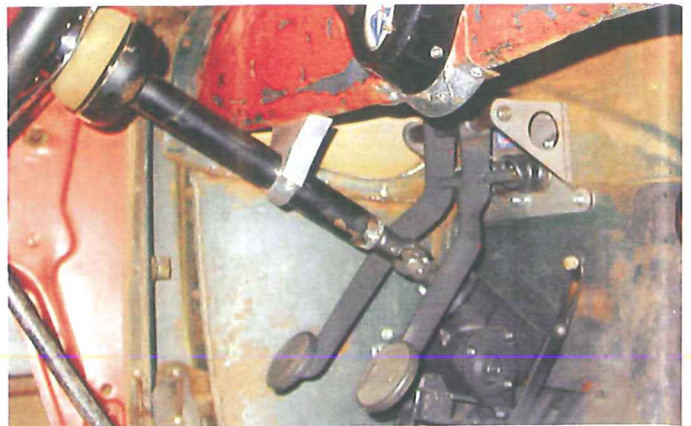
Once I got the pedals and pushrods installed into the bracket I again switched gears and went back to the steering box bracket. When I got that reinforced and solid enough to resist the torque generated when turning the wheels I then fashioned a shorty column using a '40 Ford steering shaft, the upper third of a column tube from a '60 Ford pickup, a swap meet find column drop, and a Grant four-spoke wheel.
