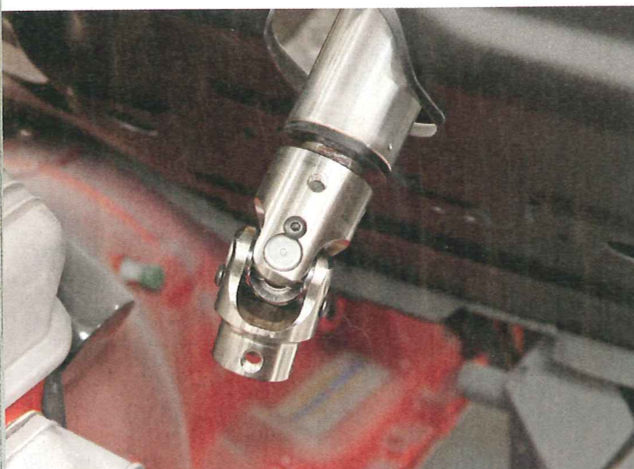
The first step in mating the column to the rack begins at the end of the column itself. Here, a 1-inch DD x 3/4-inch DD U-joint is used.
