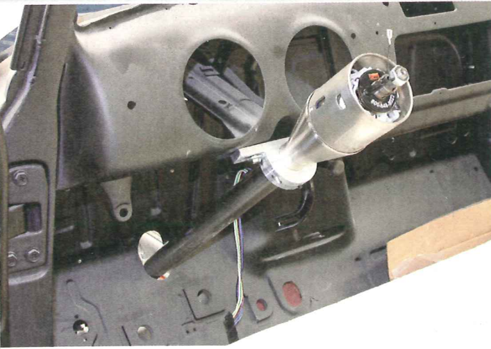
Here's our Flaming River tilt column installed in the stock location using their OEM factory-style dash mount clamp.
