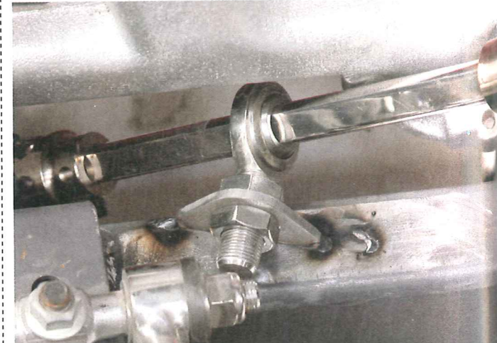
A simple bracket is fabricated and tack-welded to the chassis to mount the support bearing. The support bearing prevents the linkage from binding due to the three U-joint setup.
