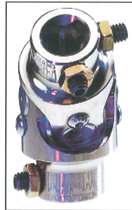
14 For an easy, safe installation, U-joints are available with splines or double-D. In most cases the maximum safe working angle of a single U-joint is 35 degrees.
