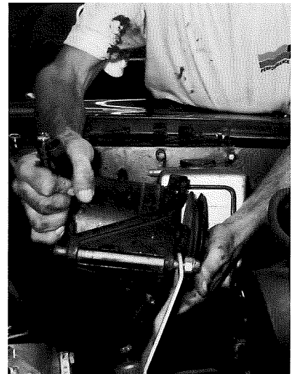
7 If your car has power steering, remove the pump from under the hood.
