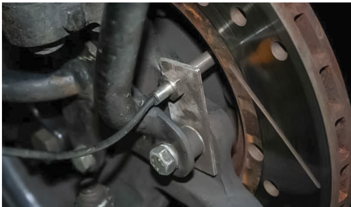
SENSOR MOUNTED ON BRAKE DISC
