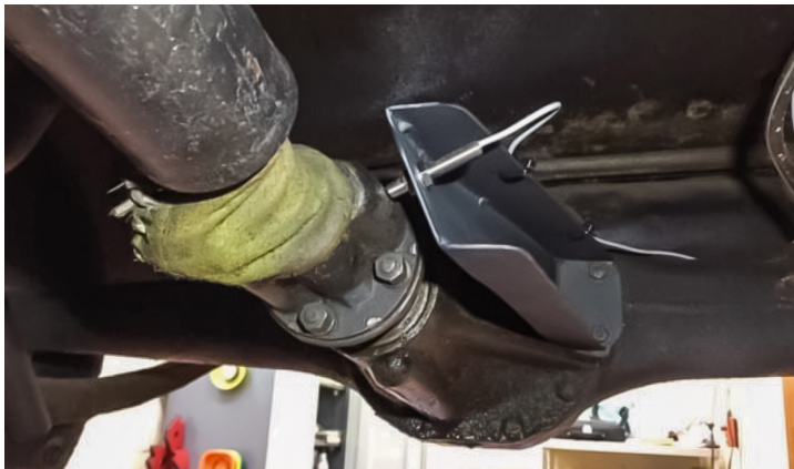
SENSOR MOUNTED ON PROPELLER SHAFT
