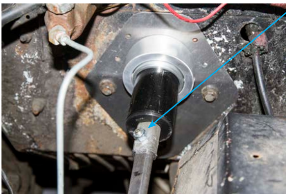
DRILL 5/16" HOLE AND INSERT BOLT
