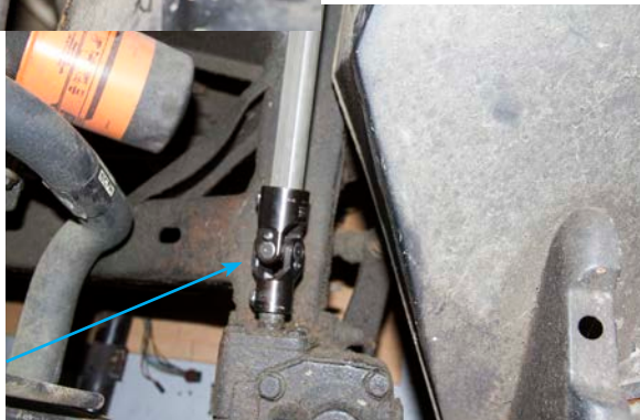
U-JOINT INSTALLED ON BOX AND SHAFT
