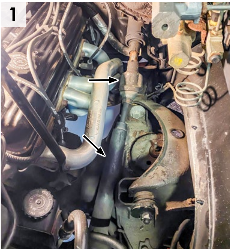
1 Disconnect and remove the factory intermediate shaft.
