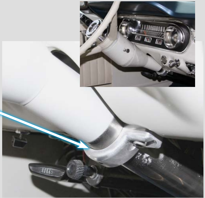
FR20114FD – 1965-70 Mustang Dash Mount Clamp – (Satin) FR20114FDPL – 1965-70 Mustang Dash Mount Clamp – (Polished)
