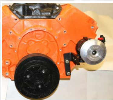
Install pump to bracket (2) using bolts (9) and washers (10) supplied
