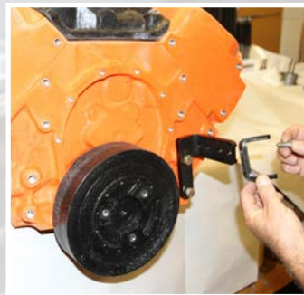
Install pump bracket (1) to L-shaped bracket (2) with bolts (15) and washers (13) supplied
