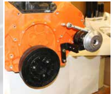
Remove upper water pump bolt. Install spacer (6) and adjuster with bolt (7) and washer (8) supplied
