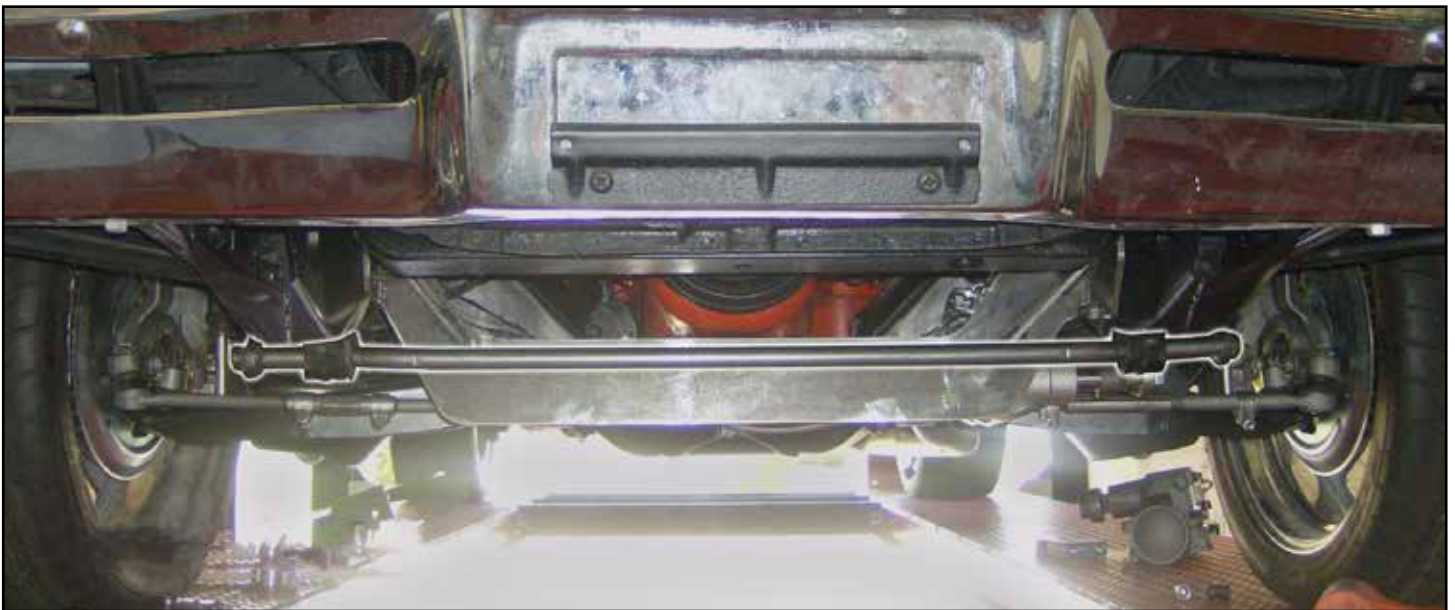
New Sway Bar Installed in Car
