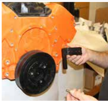
Install L-shaped bracket (1) on engine with bolts (15) and lockwashers (11) supplied
