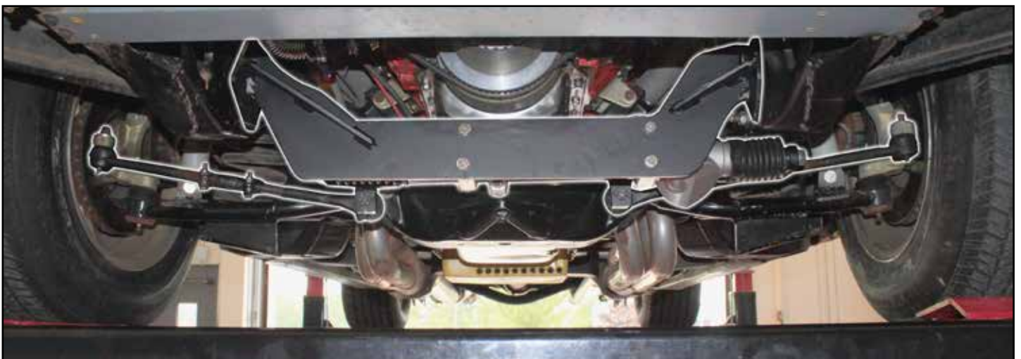
Rack & Cradle Installed in Car
