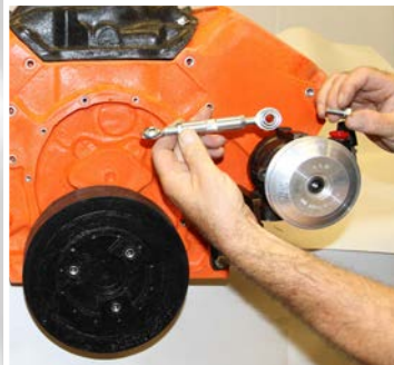
Install adjuster to pump using bolt (9) and washer (10) supplied
